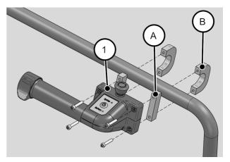
To comply with the specifications as per the IPX4 protection class, observe the horizontal installation position shown below.
