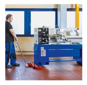
The newly developed wheel has four ball bearings and consists of a toothed aluminium core that is encapsulated with polyamide. The interlocking of the core and the tread is crucial. It provides a larger connection surface and at the same time ensures that the two components interlock.
