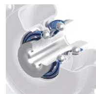
Cone ball bearing provides improved rolling properties.
